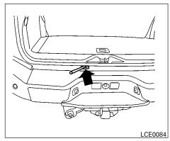
4. Assemble the two straight pieces of the jack rod. Find the oval-shaped opening above the middle of the license plate. Pass the T-shaped end of the jack rod through the opening and direct it toward the spare tire winch, located directly above the spare tire.
